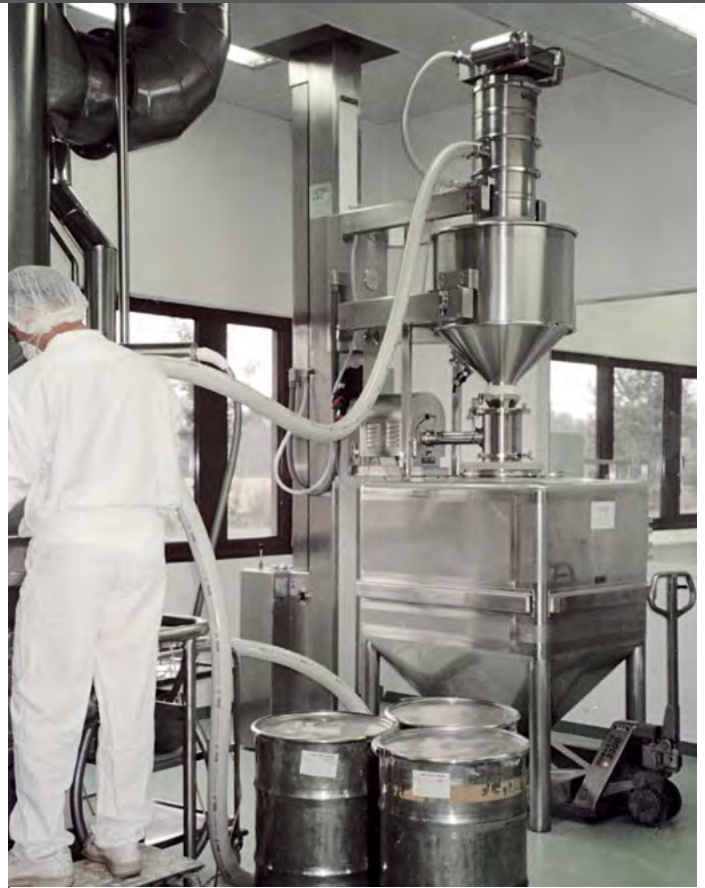
Emptying a dryer with a manual suction wand.
