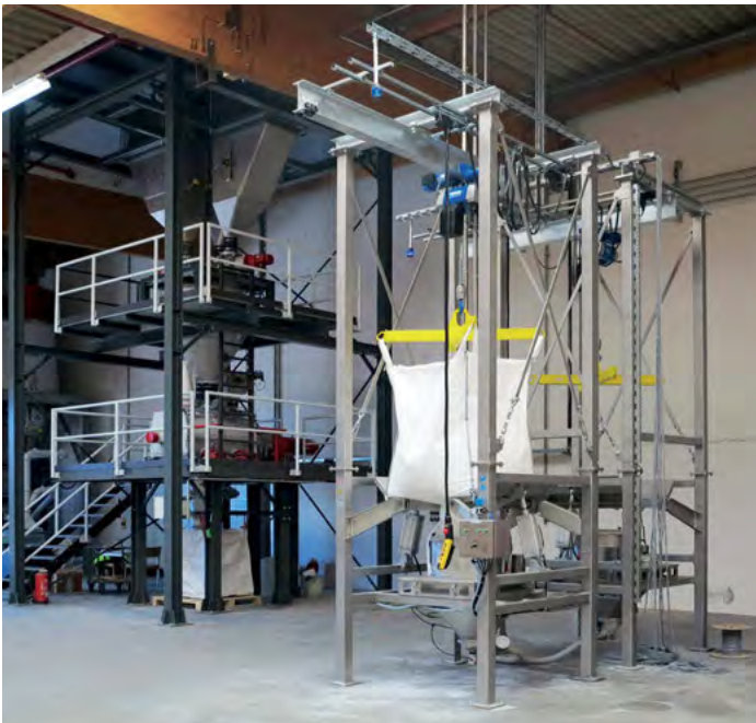
Big-Bag discharging station for conveying of various powders (some are abrasive) into a mixer.
