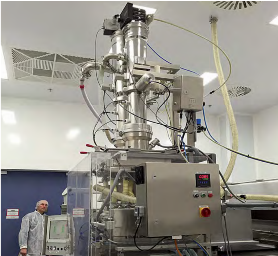
Feeding of two different powders (active pharmaceutical ingredients) into a stickpack packaging machine.
