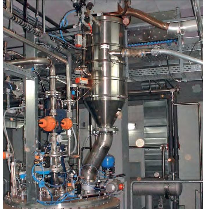
Vacuum conveyor with a powder lock for conveying pigments in a solvent atmosphere.
