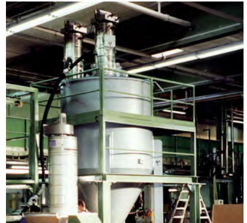
Continuous charging of a mixing container and autoclave for manufacturing adhesives.
