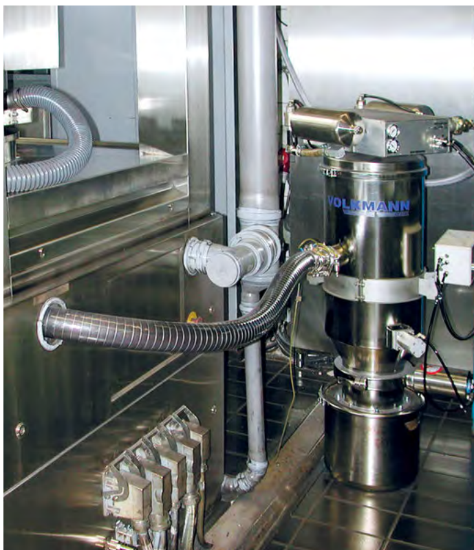
The dust, that occurs inside the tablet press during the pressing, is picked up by an industrial vacuum conveyor
