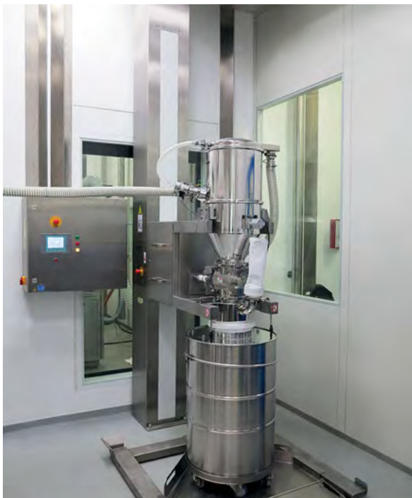
PPC 350VS with rotary valve dosing active substances.
