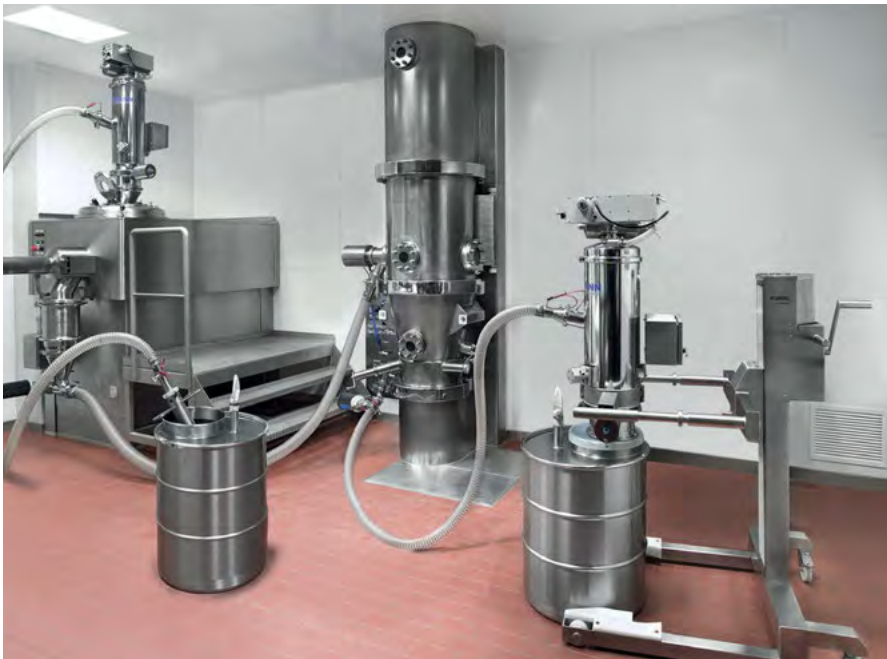
Emptying the drum and loading the mixer; Emptying a fluidized bed dryer and filling the drum.
