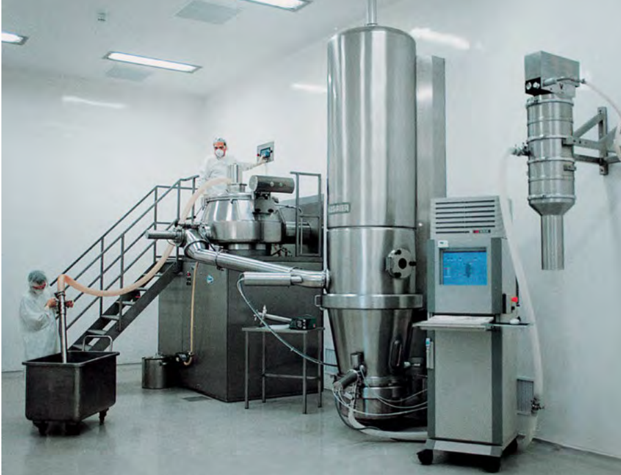
Vacuum conveyor for automatically emptying a fluidized bed dryer. Product is dispensed via an immersion pipe into IBCs.
